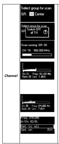
Once started a channel scan operation the receiver asks for group to be used\*. Press the SEL button to select the group to scan.
