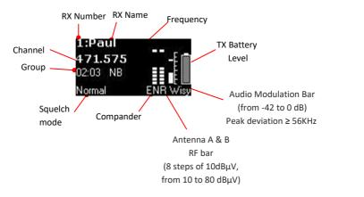
From the single receiver page press SEL button to enter direct into the Frequency setup.
