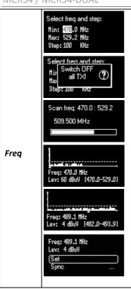
The Frequency scan allows to select a range of frequency to scan, between a maximum and a minimum value and the step with which to perform the scans. Press and hold the SEL button to confirm.
