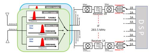
For each antenna the RF signal is split in 4 to receiver 1,2,3 and 4 (antenna A and antenna B) with a wide band splitter. Then 3 banks of filters are selected according to the frequency of the 4 receivers:
