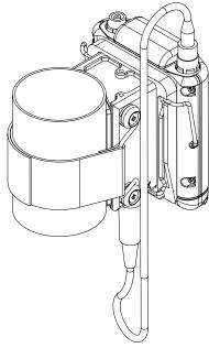
5. connect the CAL48S cable from the LEMO connector of the MTP60 to the TX connector (TA5)of the PHA60
