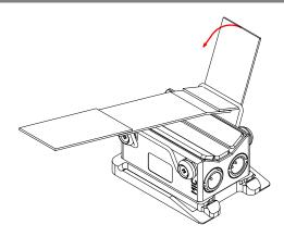
1. insert the felt on the first spring and fix the felt on one side
