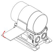
2. pass the felt around the pole and secure it on the other end
