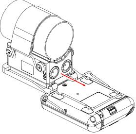
3. mount the MTP60 fixing it with the clip as shown in the figure
