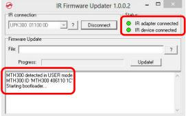
wait that both leds on the Status Panel become green and check in the lower box that the transmitter are in bootloader mode 7. Click on button in the Firmware Update panel and select the .WFU file (see step1)
