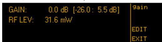
with gain = 5,5dB (max) →  $P_{\text{ampl}} = 112.2\text{mW}$
