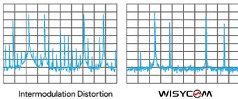
**Evenly Spaced Frequencies** - The #1 benefit of IMD Phase Cancellation is the ability to utilize evenly spaced frequencies (Wideband Channel Filters with 400 kHz min. spacing) for more channels with no intermod issues.
