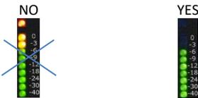
the MOD. (modulation) bar shows the MAXIMUM NUMBERS OF GREEN LED INDICATORS AND NO YELLOW/RED PEAK LED INDICATOR
