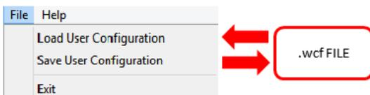
Using a file menu at the top left of the panel it is possible to **load/save all the configuration** values of the device to/from a .wcf file (Wisycom Configuration File).
