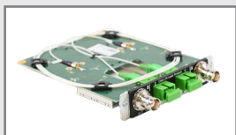
Item: EX3 expansion board version 3 (Fiber)
