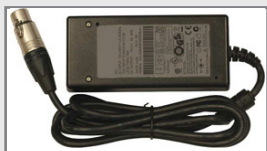
Item: AL1265XF AC/DC Power Supply with XLR-F 4-pin connector Input: 90 ÷ 264 Vac Output: 12V/5.8A supplied by default with the rack
